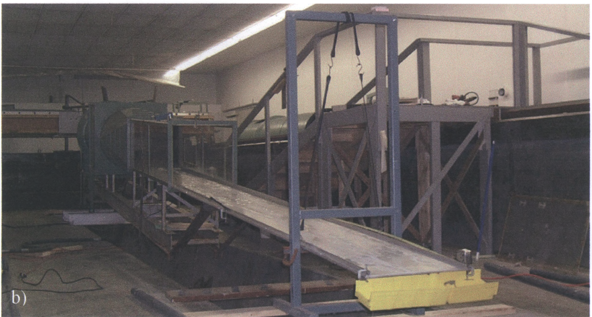
Figure 3.7 Photos of the icing windtunnel configured for rivulet-flow experiments.
