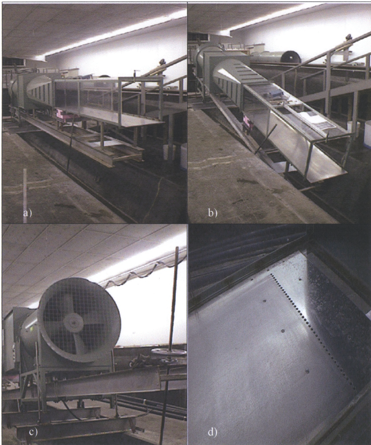
Figure 3.6 Photos of the icing windtunnel configured for sheet-flow experiments.
